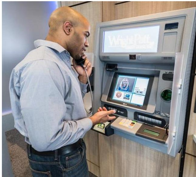
**Figure 3 - A customer using an NCR ITM. Note the video conferencing equipment, the signature pad on the lower-right, and the ID scanner on the lower-left.<sup>15</sup>**
